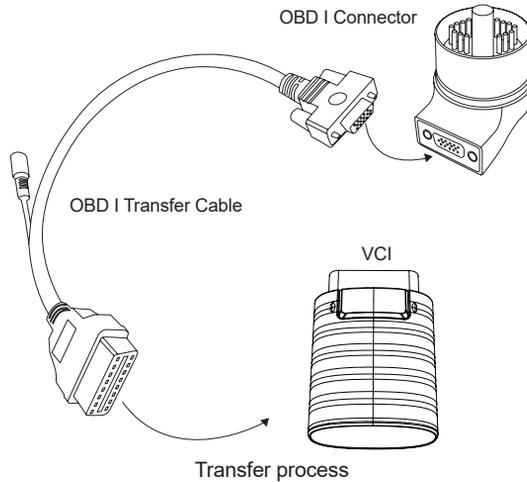
⚠ Note: when using older models, the Transfer Cable must be used, with the small power connector on it, which is connected to the power connector of the power double clamp cable, this is a solution for certain cars before 1996, whose diagnostic holders do not have a 12V power supply.
