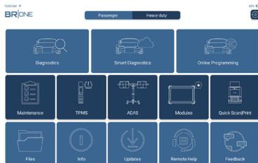
If the device failed to access the VIN information, please use "Diagnostics". At this point, you need to manually input the VIN code to gain the car information.
