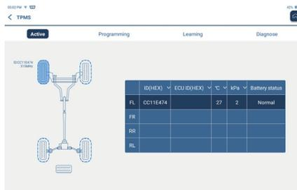
B. Programming: to program sensor data to a new BREININGER GmbH sensor, so as to replace a sensor that is in low battery and does not function properly. There are three sensor programming methods
